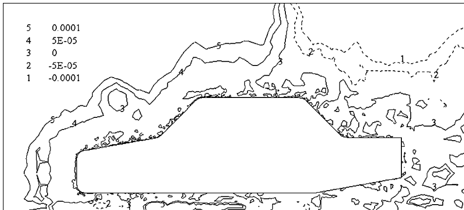
Figure 20. Instantaneous distribution of the dynamic LES model constant near the surface of the MIRA model.
